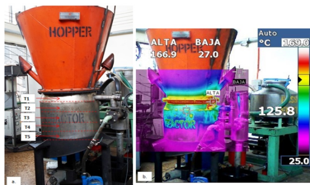
Figs. 4. (a) Temperature measurement placement along the reactor and (b) thermography of this vessel under stable conditions
