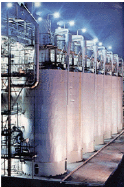
Figure 1. MSG production fermentors. The volume of each is 63,420 gallons and the height is about 100 ft tall. Hofu, Japan. (from http://smccd.net/accounts/case/biol230/indfer.html )
